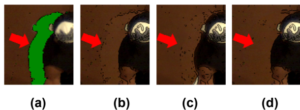
Figure 8. Color mismatch is reduced by the proposed color compensation. (a) virtual view with un-filled occlusion, (b) occlusion filled by [8], and (c) VSRS, (d) occlusion filled with proposed color compensation. The dark lines are the edge filter result to highlight the color mismatch boundary.
